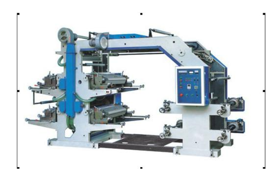
The printing machine uses the photopolymer plate .lt is suitable for the printing on the non-woven fabrics, PE, polypropylene plastics web etc.
